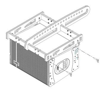
Step 3 - Insert a locking pin on both front swivel arms first, then lift the frame at the back until the swivel arm is aligned with the  $0^{\circ}$  hole. Insert now lock pins at these holes on both sides of the element and verify they're secure.
