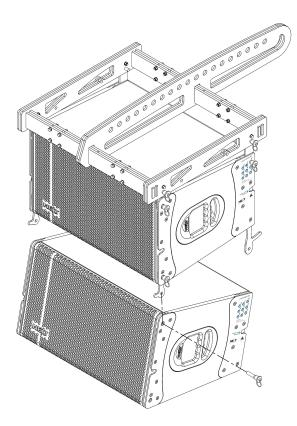
Step 5 - Insert the next LA122 $_{v2}$  in the array starting with the front side and insert the front locking pins. Check if the locking pins are secured.
