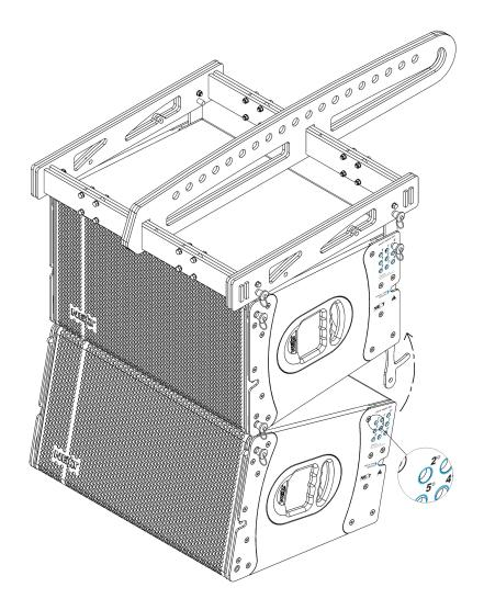
Step 6 - With the front swivel arms locked in place you can now rotate the element and with the aid of the handles on the rear swivel arms lock the element with a splay angle of 2°. Insert the locking pins and check that they are secured.
