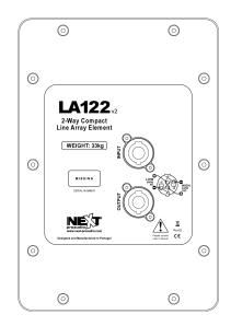
The 4 pins of the two Neutrik® NL4 SpeakON® sockets are wired in parallel within the enclosure. Either connector can be used to connect to the amplifier or another LA122v2/LA122Wv2 element. Please notice that LA122v2/LA122Wv2 Line Array element is a two-way system. See the table and the diagram below:
