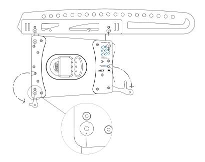
**Step 4** - Pull the LA122<sub>v2</sub> swivel arms out. On the front swivel arms, insert the locking pin. This will assure that the centre of rotation of the next element is fixed. Check if the locking pin is secured.
