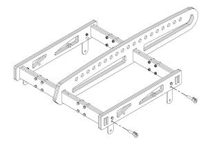
Step 1 - Pull the frame's swivel arms out of the parking position and insert a safety locking pin in each swivel arm locking position as shown in the image above. Verify that the locking pins are secured.
