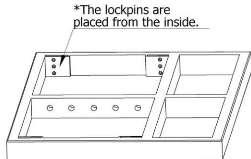
2. Insert the front joints on the frame on hole (a) and place two lockpins.
